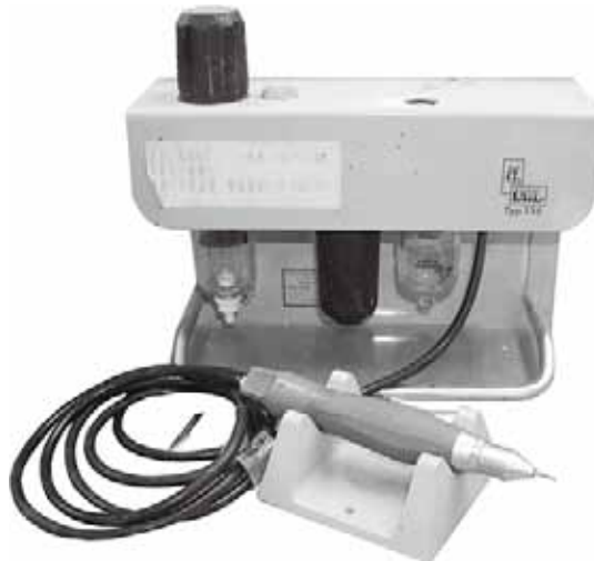
▲ Figure 2-13 Air turbine
